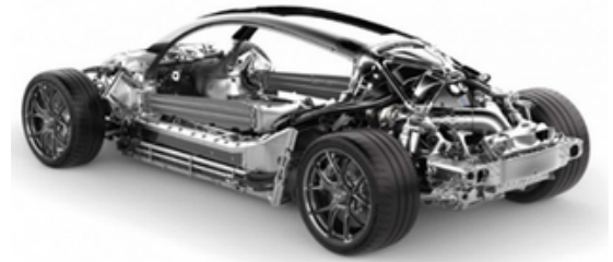
The Chassis of the 21C designed by the Czinger A.I. A chassis is the base frame of the car.
