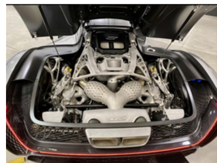
The Engine Bay of the Czinger 21C showcasing its 3D printed components.
